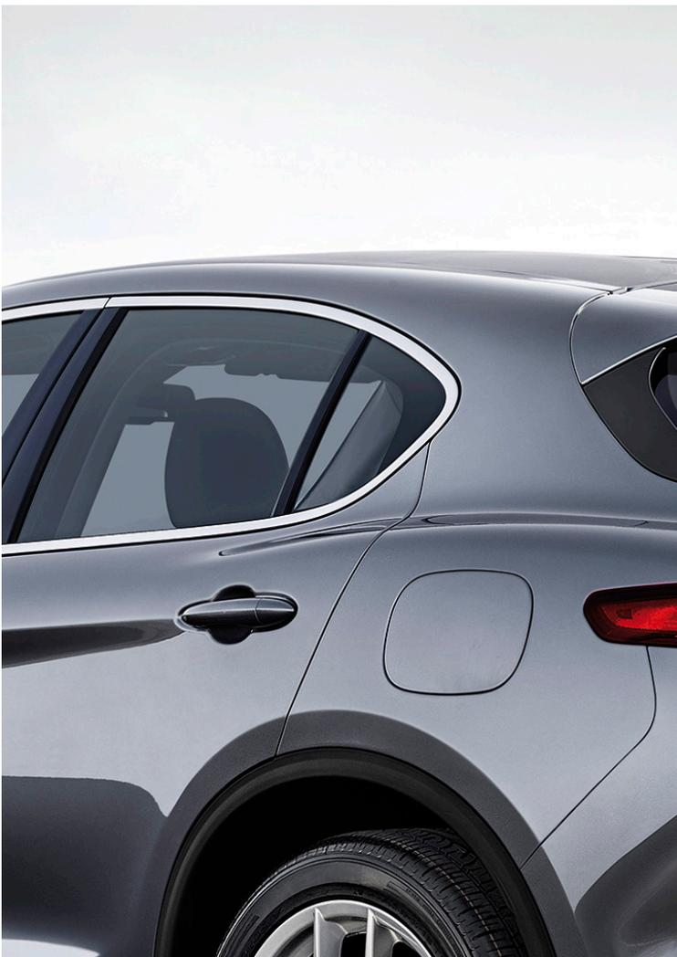
5505 and 55AT alloys have been developed by Aludium specifically for exterior automotive trim applications. These include window frames, roof rails, sunroof trim, roof racks, B- and C-pillar decoration, and other exterior decorative parts which require the highest quality finish.
